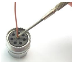
b. Push with tools when the cable is too thin.
