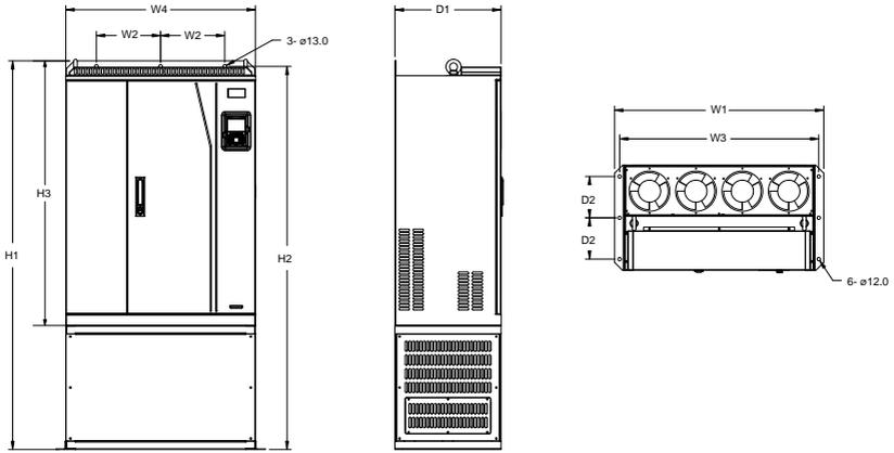
Figure C-12 Outline and mounting dimensions of 660V 400–630kW VFD models
