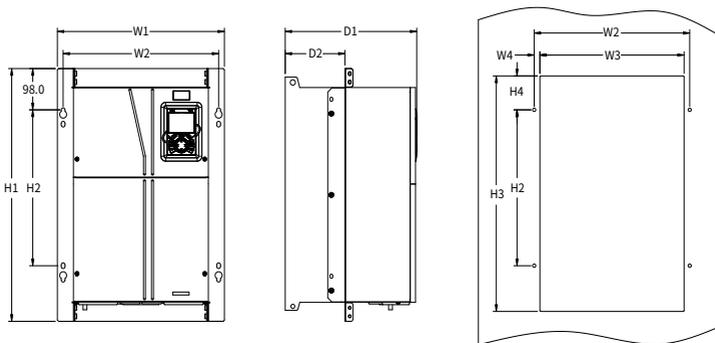
Figure D-5 Flange mounting dimensions and hole spacings for VFDs of 380V 132–200kW
