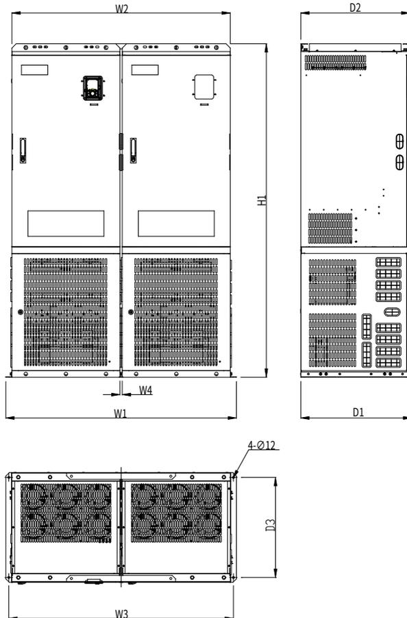
Table C-4 Parallel outline dimensions and mounting holes of 660V VFD models
