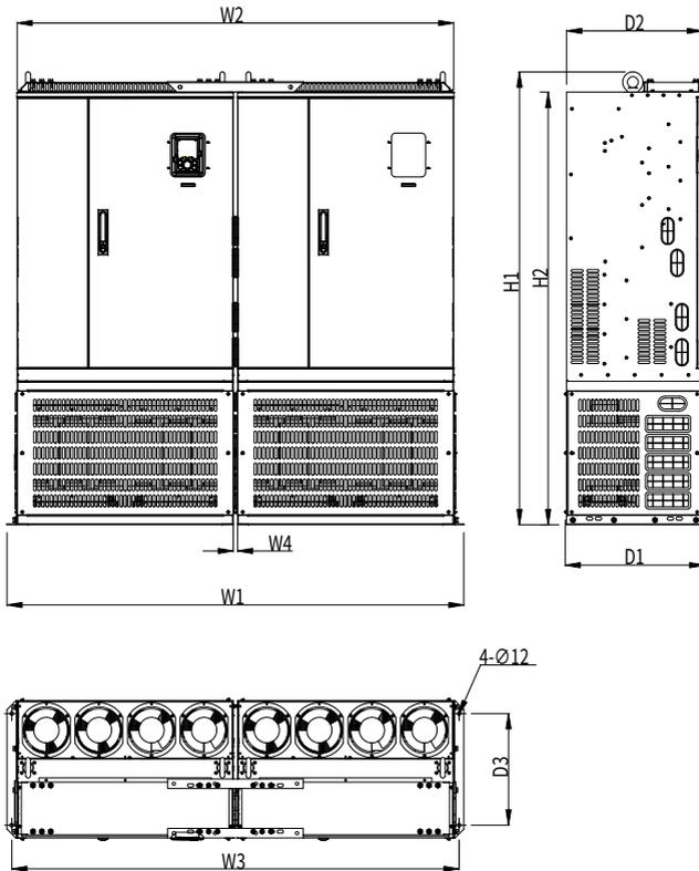
Figure C-16 Parallel outline and mounting dimensions of 660V 800–3000kW VFD models
