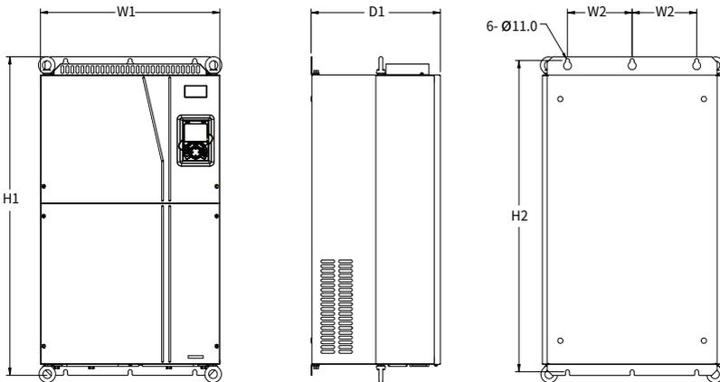
Figure C-11 Outline and mounting dimensions of 660V 250–355kW VFD models
