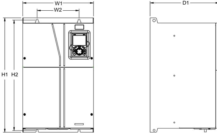
Figure C-5 Outline and mounting dimensions of 380V 132–200kW VFD models
