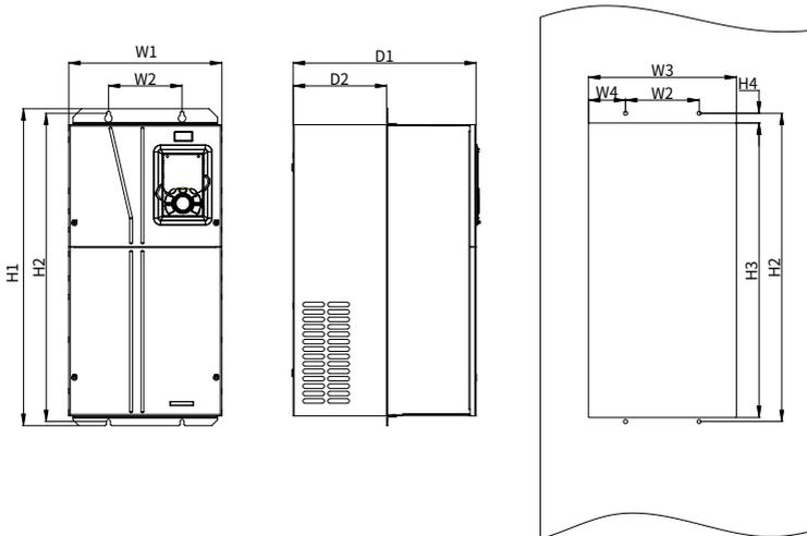
Figure D-7 Flange mounting dimensions and hole spacings for VFDs of 660V 55–132kW
