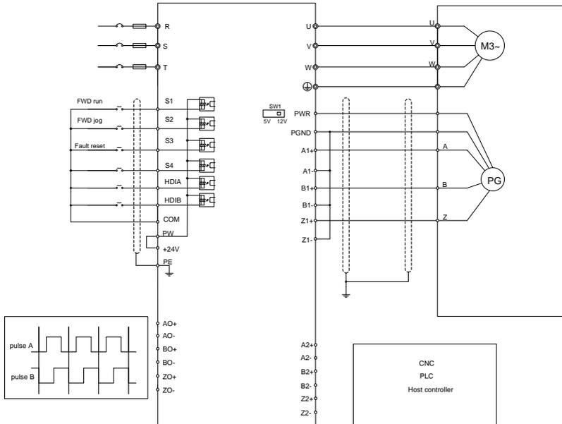
Figure E-24 External wiring when used with a push-pull encoder
