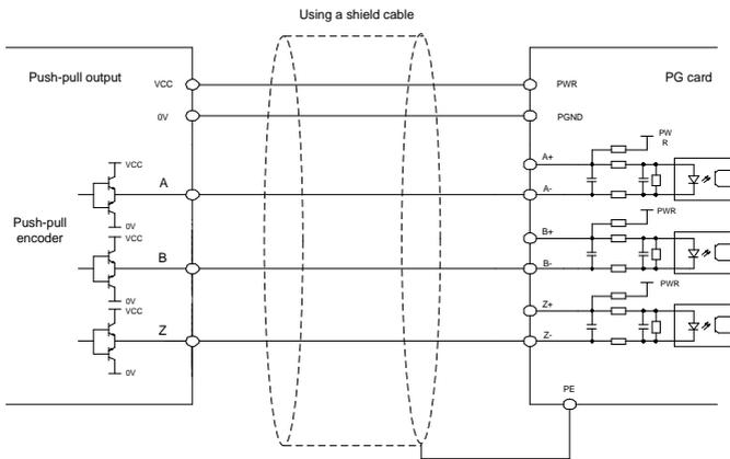
Figure E-33 External wiring when used with a differential encoder
