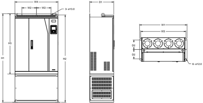
Figure C-7 Outline and mounting dimensions of 380V 355–500kW VFDs
