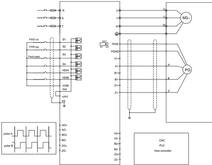
Figure E-25 External wiring when used with a differential encoder
