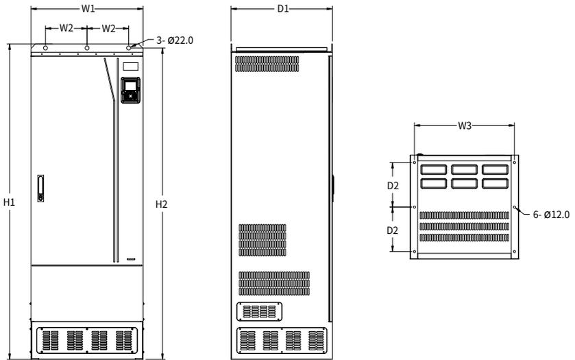
Table C-1 Outline dimensions and mounting holes of 380V VFD models
