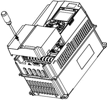
Step 2 Use a tool to pry up the snaps on both sides of the lower cover. Lift up the bottom of the lower cover gently and take out the lower cover.
