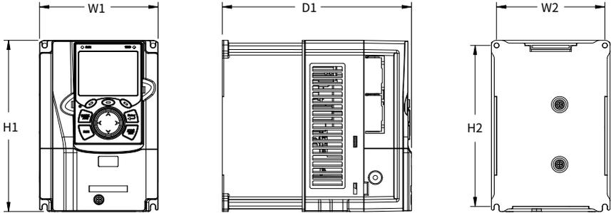
Figure C-3 Outline and mounting dimensions of 380V 45–75kW VFD models
