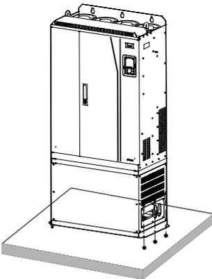
**Step 2** Fix the VFD on the ground or mounting plate, and tighten the screws on the ground or mounting plate.
