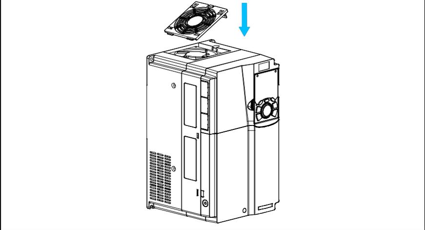
**Disassembling a fan (380V 90–500kW, 660V 110kW or higher)**
