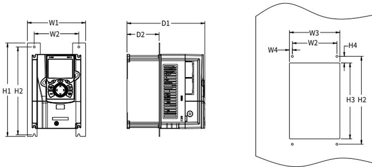
Figure D-4 Flange mounting dimensions and hole spacings for VFDs of 380V 90–110kW
