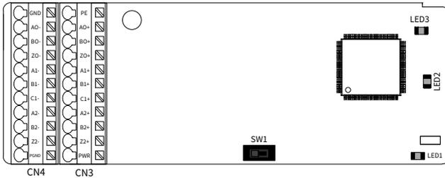
SW1: the switch used to set the voltage class (5V or 12V) of the power supply of the encoder. It can be operated with an auxiliary tool.
