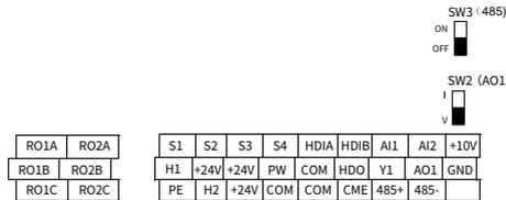
Figure 4-8 Terminal diagram of the 7.5kW and higher control circuit
