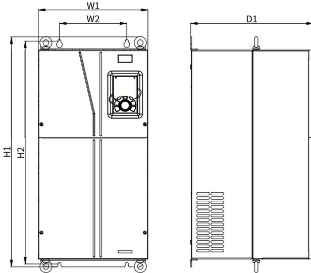
Figure C-10 Outline and mounting dimensions of 660V 160–220kW VFD models
