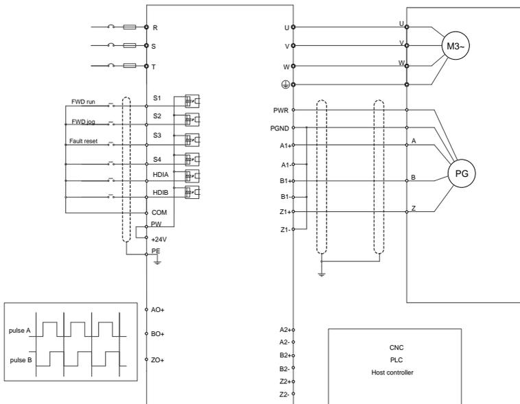
Figure E-28 External wiring when used with a push-pull encoder
