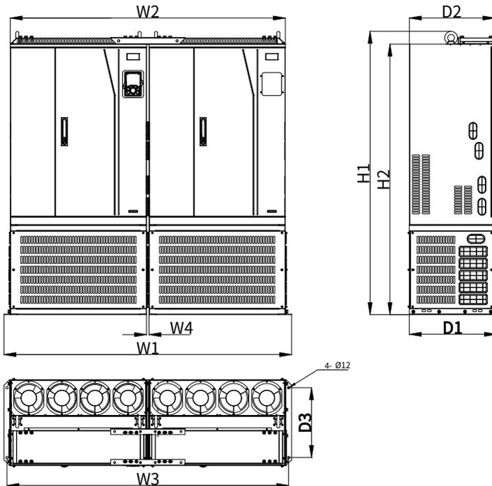
Figure C-14 Parallel outline and mounting dimensions of 380V 710–3000kW VFD models
