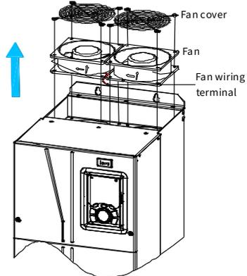
**Assembling a fan (380V 90–500kW, 660V 110kW or higher)**
