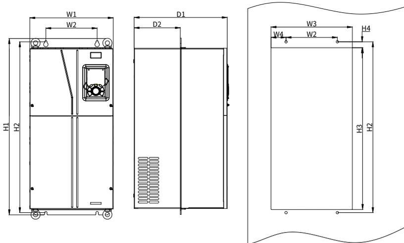
Figure D-8 Flange mounting dimensions and hole spacings for VFDs of 660V 160–220kW
