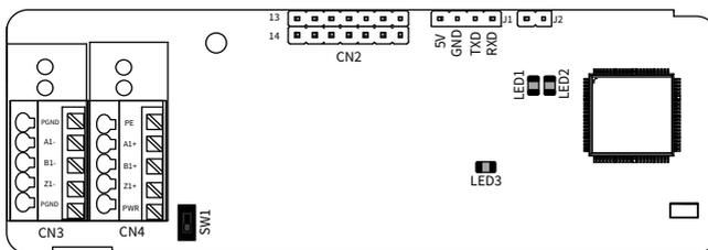
SW1: the switch used to set the voltage class (5V or 12V) of the power supply of the encoder. It can be operated with an auxiliary tool.
