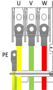
Step 3 Connect optional parts such as the braking resistor that carries cables to designated positions. For details, see 4.3.1 Main circuit wiring diagrams.
