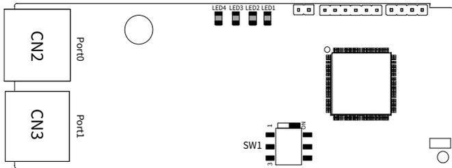
**Note:** For this card, before power-on, set the SW1 switch according to the mapping between protocols and positions.
