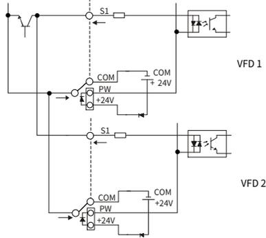
Method 2: If the input signal comes from the PNP transistor, set the U-shaped jumper between COM and PW based on the power used according to the following figure.
