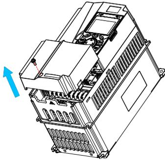
Step 2 Unscrew the screws in the middle of the housing and remove the upper cover.
