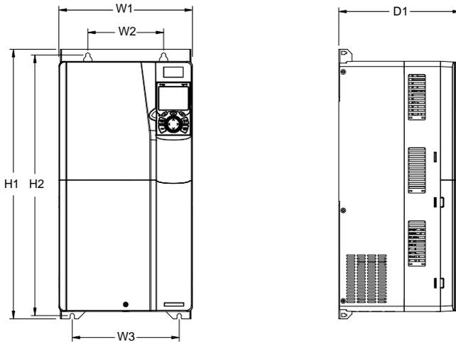
Figure C-4 Outline and mounting dimensions of 380V 90–110kW VFD models
