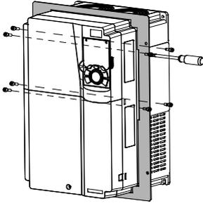
**Step 2** Fix the VFD with bracket on the control cabinet, and tighten the screws on the front of the bracket.
