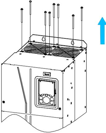
Step 2 Take out the fan cover and fan, and remove the fan connection terminal.
