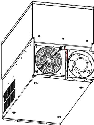
Step 2 When putting the fan and fan cover into the mounting place, align the mounting holes with the fixing holes, and fasten the screws.
