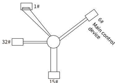
Use shielded cables, if possible, in multi-device connection. The baud rates, data bit check settings, and other basic parameters of all the devices on the RS485 line must be set consistently, and addresses cannot be duplicated.
