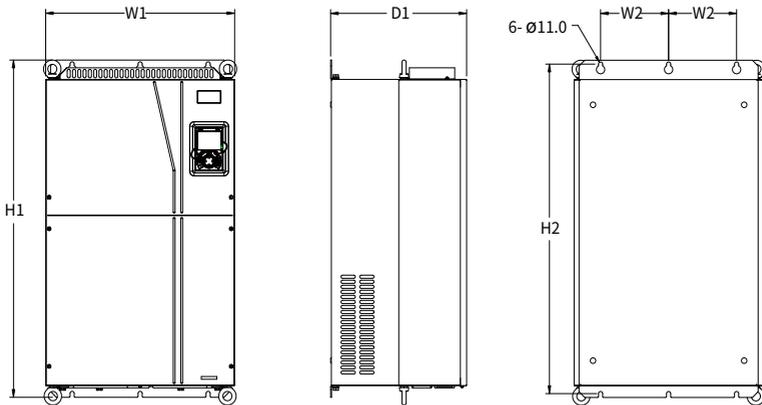
Figure C-6 Outline and mounting dimensions of 380V 220–315kW VFD models
