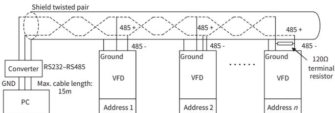
Figure 7-3 shows the star connection. When this connection mode is adopted, the two devices that are farthest away from each other on the line must be connected with a
