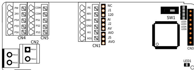
"SW1" indicates the start/stop switch of the programmable expansion card and "120" indicates 120Ω terminal resistor. By default, J1 connects to NC, J2 to AV, and J5 to AVO.
