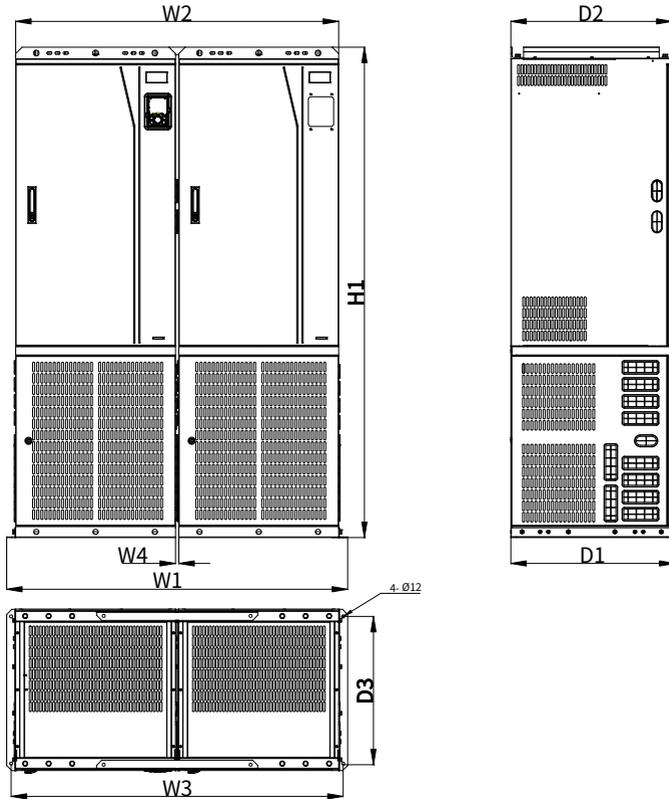
Table C-3 Parallel outline dimensions and mounting holes of 380V VFD models
