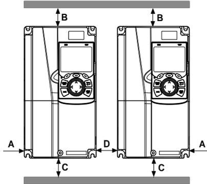
Table 3-2 Installation space dimensions of multiple VFDs
