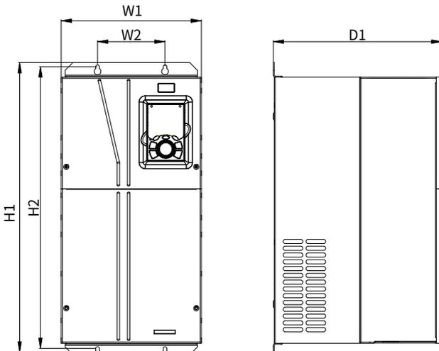
Figure C-9 Outline and mounting dimensions of 55–132kW VFD models
