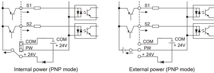
4.4.3.2 Output signal connection diagram
