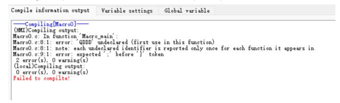
Click on "Compile Information Output" to view the compilation status, if there is an error, it will provide relevant hints as shown in the figure above. If the compilation is successful, executable macros will be
