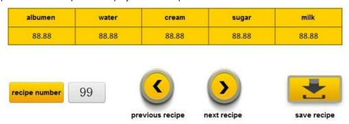
It can change recipe parameters via Numerical input and display; realize functions of checking recipe, reading recipe and writing recipe through function buttons.
