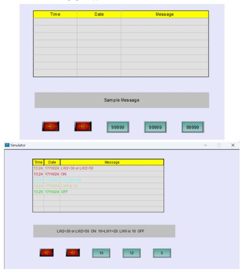
**∠Note:** Analog alarm number: at present, VS-Q series HMI can only set up 5 analog alarms.
