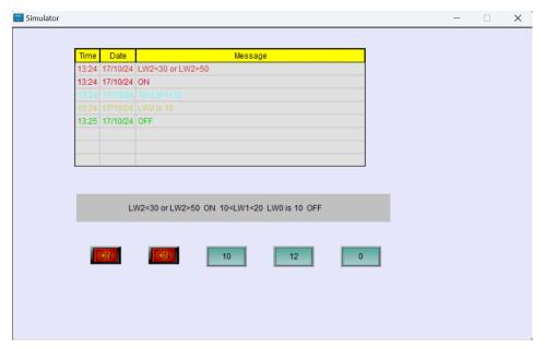
**∠Note:** Analog alarm number: at present, VS-Q Series HMI can only set up 5 analog alarm.
