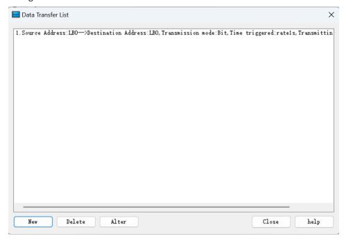
The transmission list lists details of all the current transmission items. Users can create, delete and modify them. HMITOOL configuration software supports up to 512 data transmission items.
