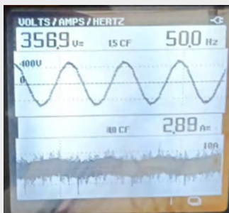
Voltage and current waveform and current distortion rate THDi after the adding
