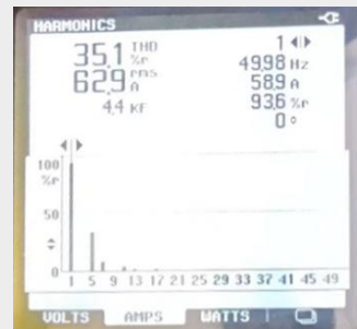
Voltage and current waveform and current distortion rate THDi before the adding
