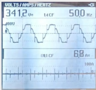
Voltage and current waveform and current distortion rate THDi before the adding
