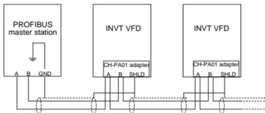
Figure 2-3 PROFIBUS bus connection
