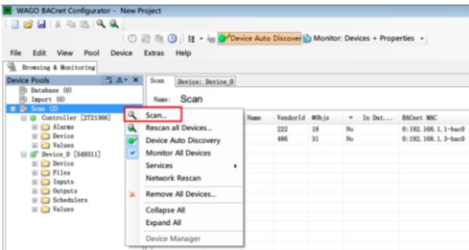
In the preceding figure, **Controller [2721366]** is the VFD node in the bus and **Device\_0 [549311]** is the PLC node. The numeric part in [] is the decimal number converted from this node MAC address.
