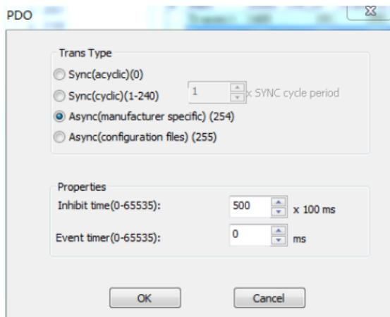
Received PDOs support all transmission modes. Generally, received PDO 1 is configured as 254 mode with an appropriate inhibition time while received PDO 2–4 are configured as synchronous mode. Different synchronous modes are configured according to real-time requirements of communication data. In the following interface, transmission mode of received PDO 1 is configured as 254, and inhibition time is configured as 50ms.
