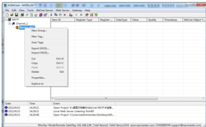
X2BACnet connects to the BACnet MSTP card through RS485. Add all scanned records, and save the project. See the following figure.
