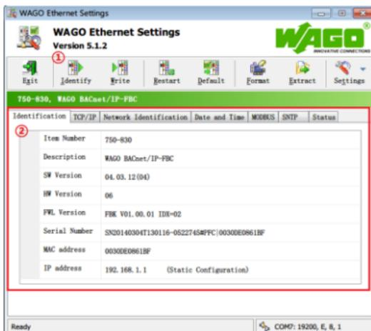
4. Click **TCP/IP** and set the PLC IP address in red box ②, and ensure the PC IP address and the PLC IP address are in the same network segment. Then click **Write** to write the set IP address to the PLC. See the following figure.
