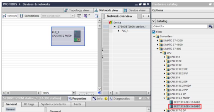
In the **Hardware catalog** pane, choose **Other field devices > PROFIBUS DP > General > INVT ELECTRIC CO.,LTD > INVT > INVT-6SE70**, and double click the **INVT-6SE70** icon or drag it to the view of **Devices & networks**. The communication card is displayed as **Not assigned**. The example shows three slave bus networking, thus you need to add two slaves.
