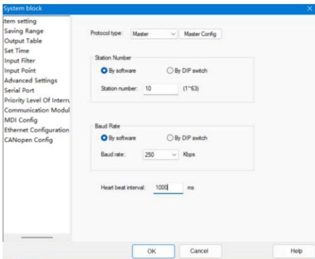
PLC station number and baud rate can be set through the software and dial-up. In this example, PLC station number and baud rate are set to 10 and 250K respectively through the software (by default).
