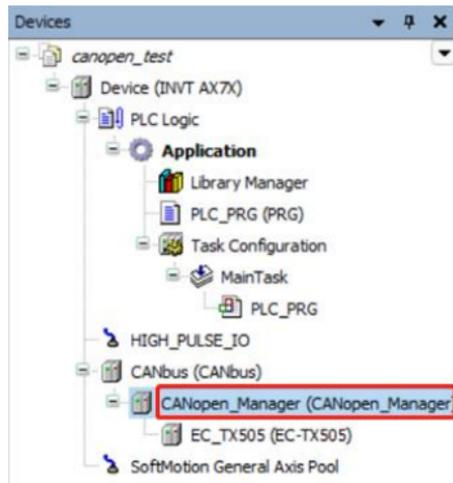
8. Double click **CANbus** in the **Devices** pane to set the baud rate of the network.
