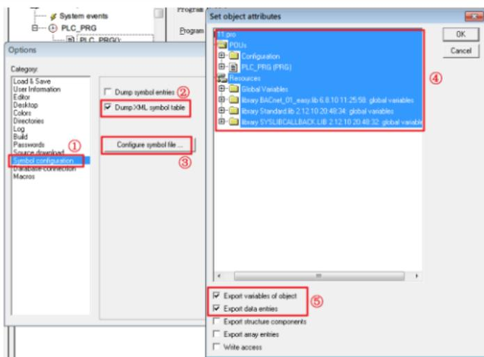
After the setup, when the POU program is completed and the PLC is in login state, the file **xxx.sys\_xml** (xxx is the project name) will be generated automatically and saved in the created project folder.
