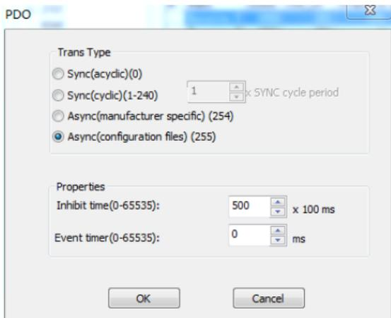
Refer to the description of CANopen communication of GD350 VFD, transmitted PDO 1 only supports 255 transmission mode, and does not support event timer mode. Therefore, received PDO 1 mode is configured as asynchronous 255 mode, and event timer is configured as 0ms, inhibition time is configured as 50ms, that is, transmitted PDO 1 message is sent at most once within 50ms.
