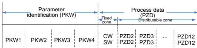
Figure 2-4 PROFIBUS-DP information frame data structure
