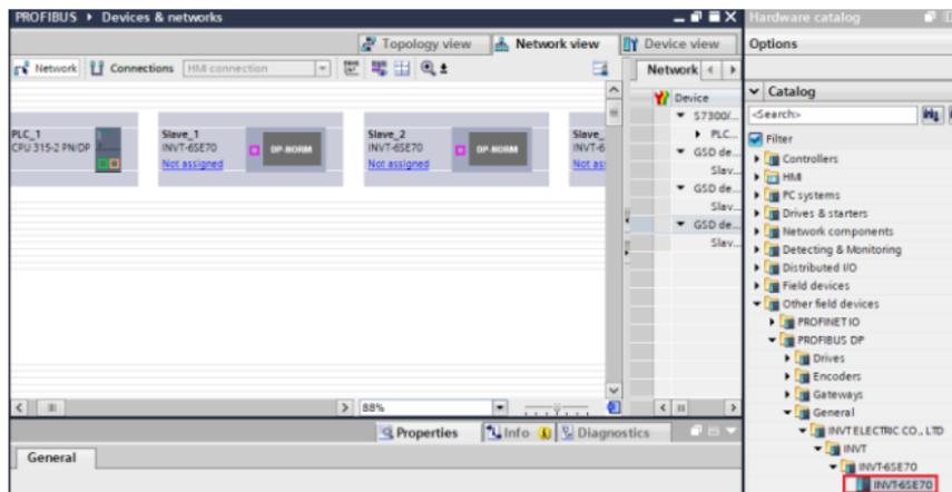
As shown in the following figure, click the **Not assigned** option of **INVT-6SE70** and select **PLC\_1.MPI/DP interface\_1**, and CPU and INVT-6SE70 in the network view are connected to the same PROFIBUS network. Click the **Not assigned** option of the remaining two PROFIBUS slaves and select **PLC\_1.MPI/DP interface\_1**, then PROFIBUS master and three slaves are connected to the same PROFIBUS network.
