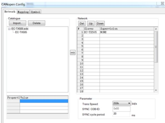
In this example, the slave number is 1, baud rate is 250k, and synchronization cycle period is 20ms.
