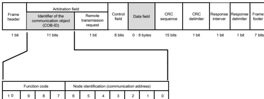
Figure 3-2 Packet structure
