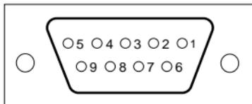
Figure 2-1 Plug of the connector
