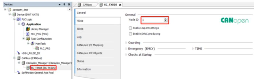
10. Double click **PDOs** in the above figure, and double click PDO mapping to set the PDO as shown in the following figure.
