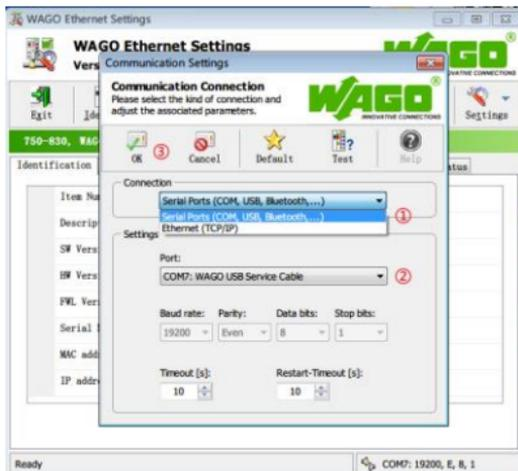
3. Click **Identify**, and wait for a while. If the PC and PLC are connected properly, the area in the red box as shown in the following figure will appear, showing information such as the PLC hardware and software versions, MAC address, and IP address. If the content in the red box area indicates that the connection has failed, check whether the connection between the PC and PLC is normal, as shown in the following figure.
