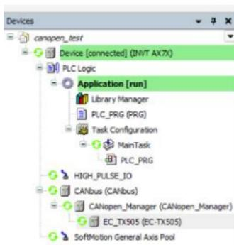
16. Open **CANopen I/O Mapping** in the EC\_TX505 page, modify the parameters of the VFD, and view the status of the VFD.
