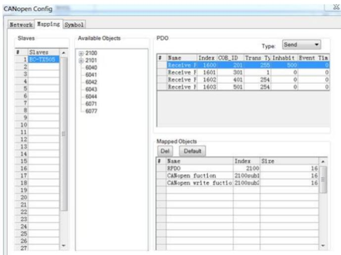
Double click one PDO to set the transmission mode, such as **sync** (mode 1–240) and **asyn** (mode 254 and 255). The interface is shown as follows.
