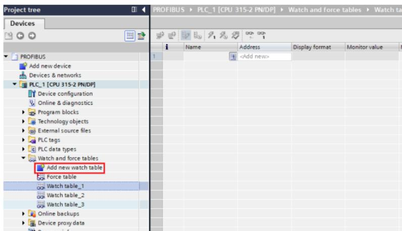
Create target watch variables—PZD, PKW, control word and status word variables of the VFD in the newly created **Watch table\_1**, and click **Watch all** and **Modify selected values at one time immediately**, as shown in the following figure. Operations in **Watch table\_2** and **Watch table\_3** are similar to those in **Watch table\_1**.
