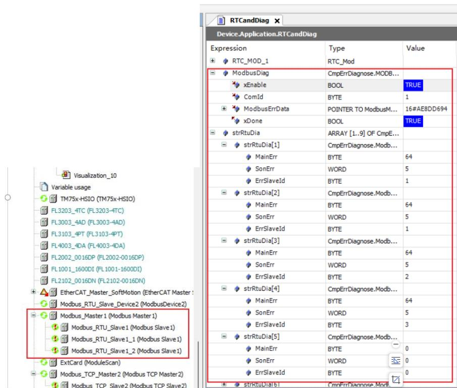
Figure 6-6 Description of Modbus Master Diagnostic Function Block Parameters
