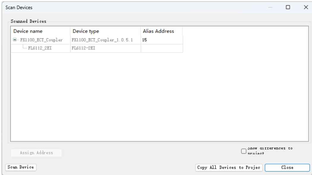
Figure 4-14 Couplers and Expansion Modules Added after Scanning
