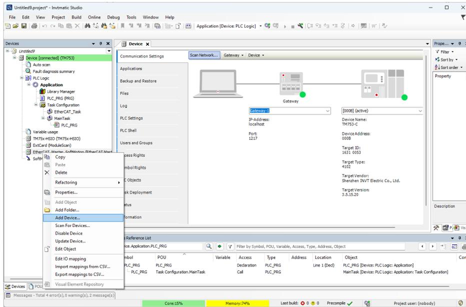
Figure 2-4 Selecting an EtherCAT Slave Device
