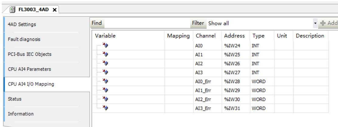
Figure 4-22 4AD Information Interface of the Analog Input Module
