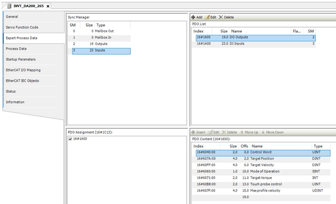
Figure 5-33 EtherCAT I/O Mapping
