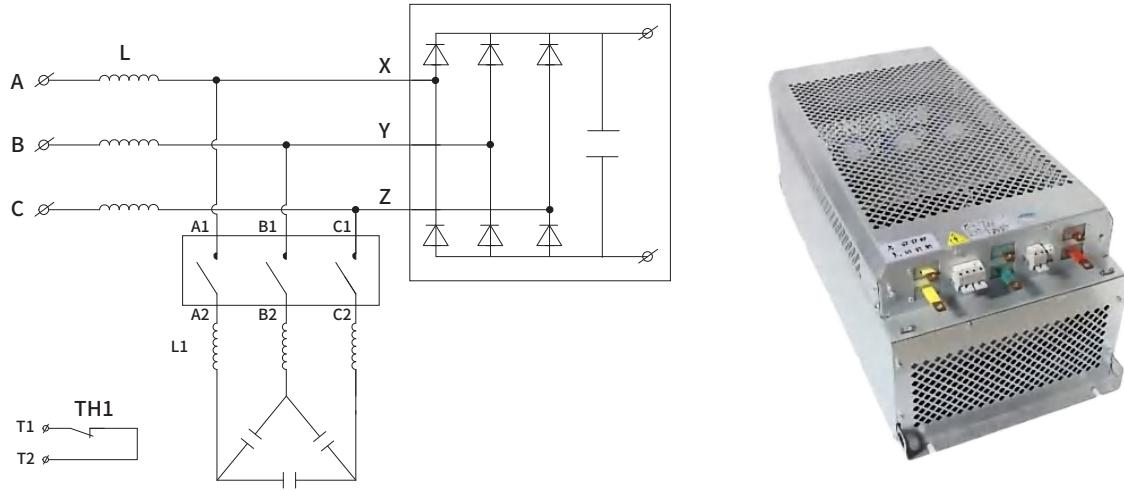
Remarks: A1A2,B1B2,C1C2, is used for connecting external contactor, factory default short connection.
