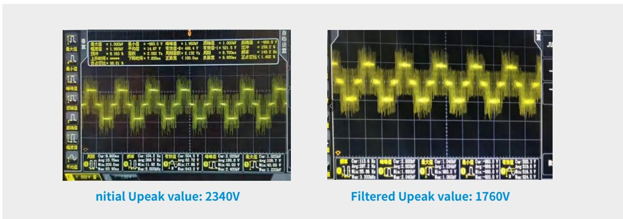
3PH-AC690V system **dv/dt values** before and after adding a **dv/dt** decrement filter
