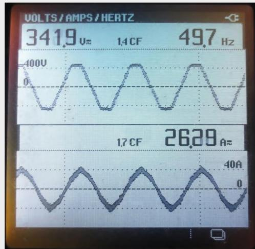
Voltage and current waveform after adding a sine filter
