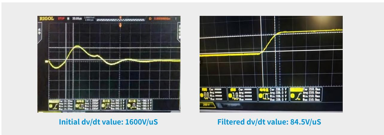
■ Comparison between dv/dt decrement filter parameters and traditional LC type dv/dt filter parameters
