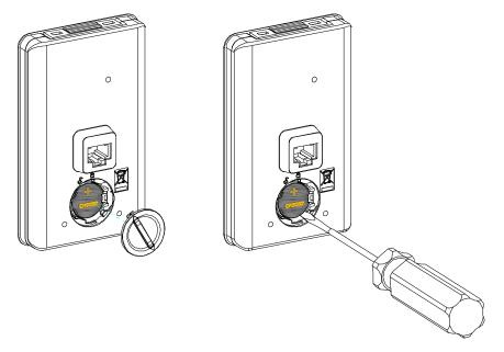
Step 3 Close the cover and rotate it clockwise by 30° to tighten it.
