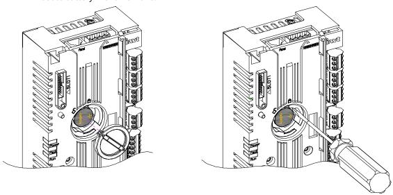
Step 3 Close the cover and rotate it clockwise by 45° to tighten it.
