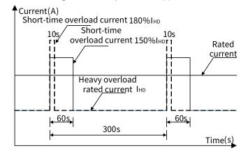
Figure 2-4 Heavy overload application
