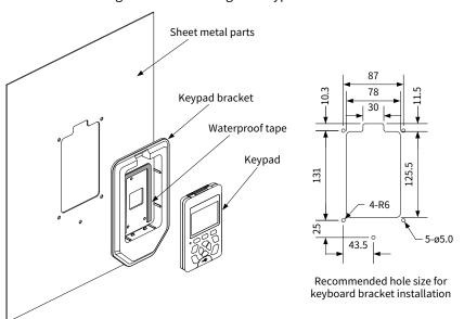
Figure 3-29 Keypad bracket dimensions (unit: mm)
