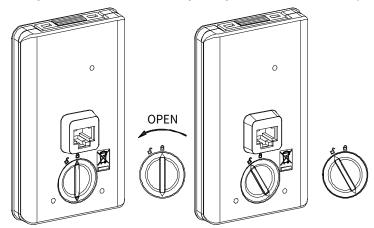
Step 2 Remove the cover, press one side of the battery with a screwdriver, remove and replace the battery with a new one.
