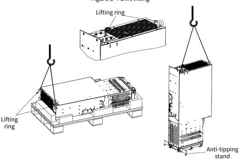
Figure 3-4 Unit lifting
