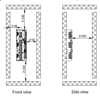
Figure 3-25 Requirements on RCU installation space (unit: mm)
