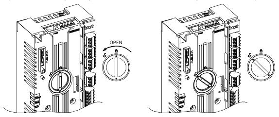
Step 2 Remove the cover, press one side of the battery with a screwdriver, remove and replace the RCU module battery with a new one.
