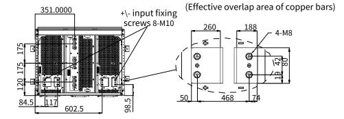
Figure B-9 Installation dimensions of A4i filter reactor (unit: mm)
