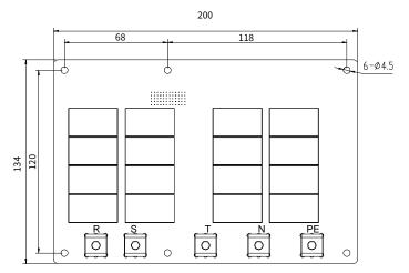
Figure 6-4 EMI filter module
