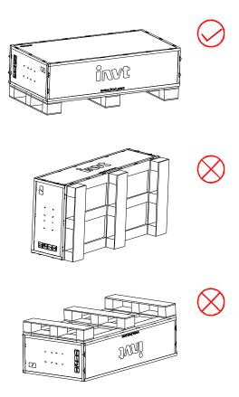
When transported with a forklift, the regenerative rectifier must be fixed to the pallets and transported together, which means you are not allowed to remove the pallets to transport the regenerative rectifier. If the forklift's fork tines are too short, it may cause the unit/cabinet to tip over, resulting in serious injury, property damage or even death.
