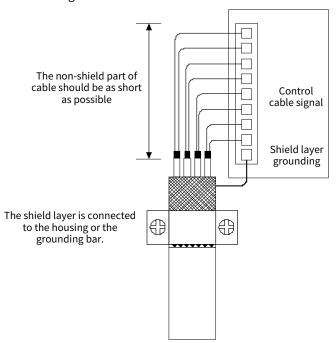
Figure 4-7 Control cable shield connection
