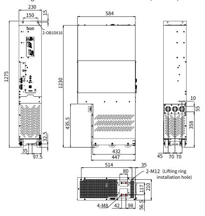
Figure B-5 Installation dimensions of A8 unit fast connector (unit: mm)
