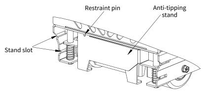
Figure 3-7 Unfolding the anti-tipping stand
