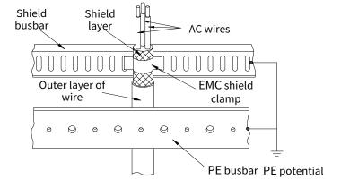
Figure 4-8 Power cable shield connection
