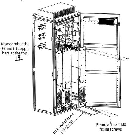
Figure 7-5 Replacement of A8 regenerative rectifier unit
