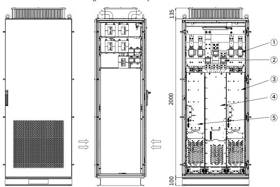
Figure 3-16 Cabinet layout for L+2\*A8
