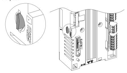
Step 2 Insert and push the SD card into the card holder of the new module in the direction shown in the figure.
