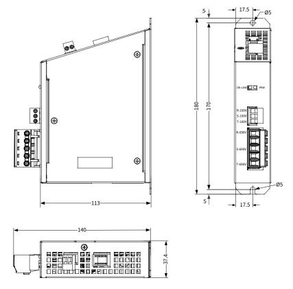
Installation of voltage detection module: The rear mounting method is used. Align the installation holes and tighten the screws.
