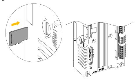
Step 3 Ensure that the SD storage card is pushed into place. Otherwise, abnormalities may occur due to poor contact.
