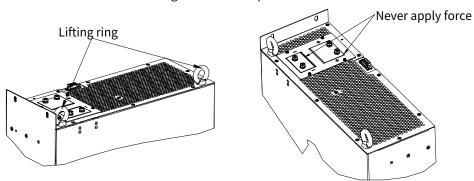
The regenerative rectifier unit has a high center of gravity and must be placed on a flat and solid ground with sufficient support strength and a tilt angle of less than 5°. Failure to comply with this requirement will cause the unit to tip over or topple over, which may result in serious injury or property damage.
