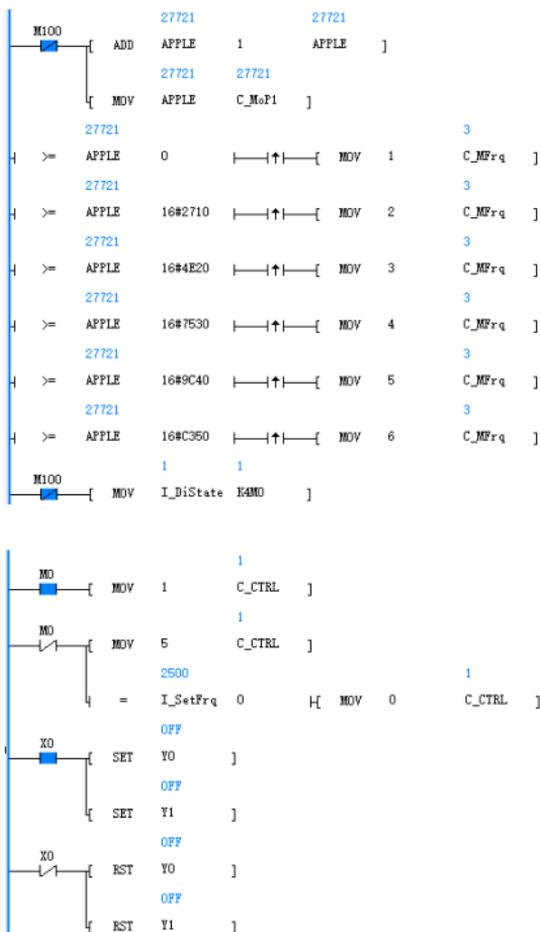
Figure 5.4 Programming case for multi-step setting and running
