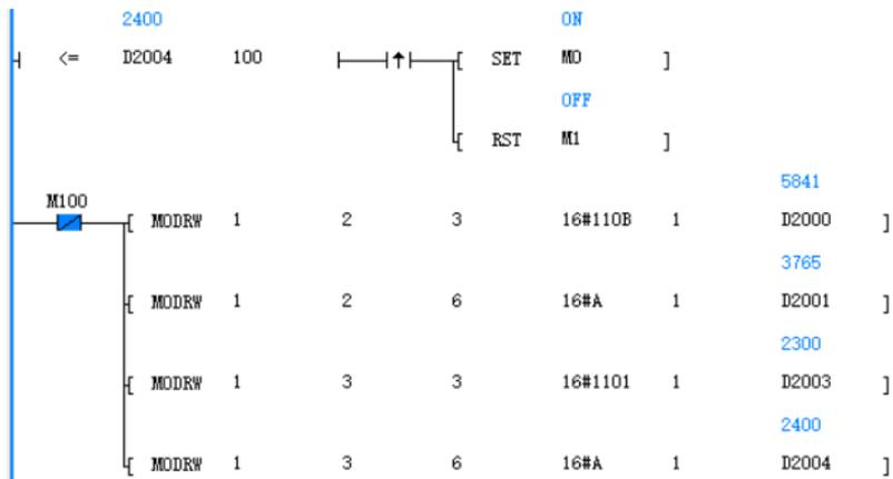
Figure 5.6 Programming case for RS485 communication
