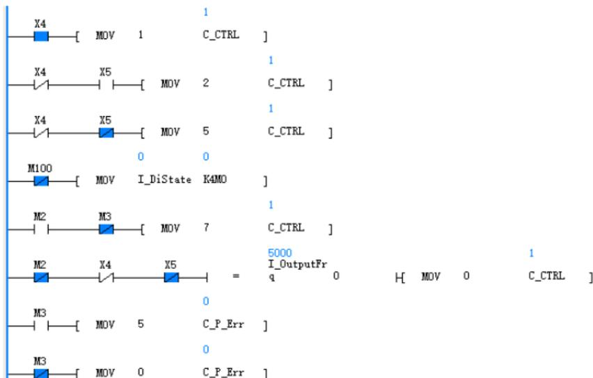
Figure 5.2 Programming case for terminal-based running/fault control
