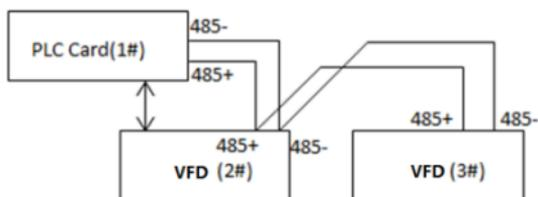
Figure 5.5 PLC card networking example
