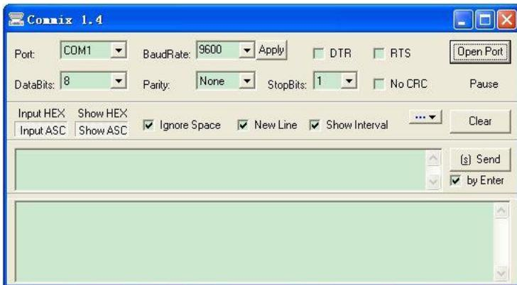
First, select COM1 for "serial port" and the baud rate should be set to the same value with P14.01. The data bit, check bit and stop bit must be consistent with the setup in P14.02. As RTU mode is used here, "HEX" should be selected. Check  ModbusRTU to make the software add CRC automatically, and select CRC16 (ModbusRTU) with the starting byte being 1. Once enabled, CRC check will be added automatically, which removes the need to fill in CRC manually.
