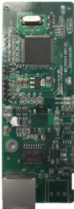
Ethernet communication card EC-TX504
