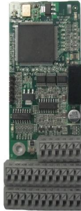
UVW incremental PG card EC-PG503-05
