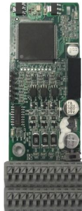
Multifunction incremental PG card EC-PG505-12
