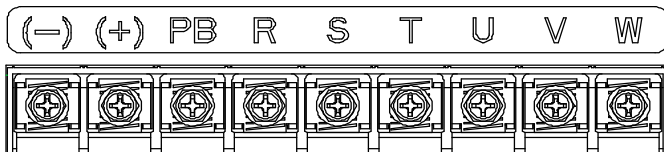
Figure 4-10 Main circuit terminal diagram for 3PH 380V 30-37kW
