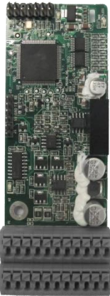
Resolver PG card EC-PG504-00
