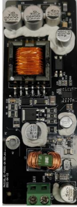
24V power supply card EC-PS501-24
