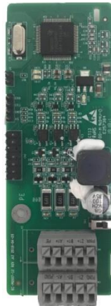
Simplified incremental PG card EC-PG507-12
