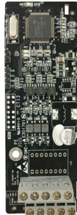
24V simplified incremental PG card EC-PG507-24
