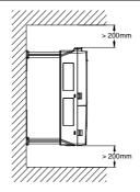
Figure 3-1 Drive installation diagram
