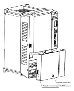
To assemble the junction box of drive (for example, MH860-T038SF7), do as follows:
