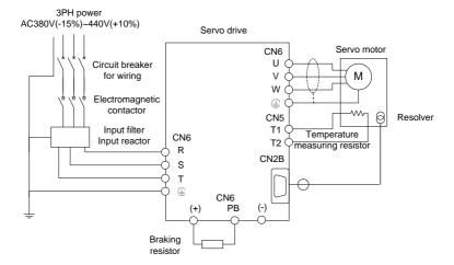
Figure 4-9 Wiring diagram of =<90kW main circuit
