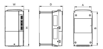
Figure 2-1 Dimensions of MH860-T018SF7-T070SF7
