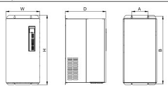
Figure 2-2 Dimensions of MH860-T092SF7-T215SF7
