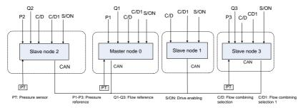
Example: The hydraulic system has four oil pumps, with the addresses set to 0, 1, 4, and 3. There may be two types of action combination:
