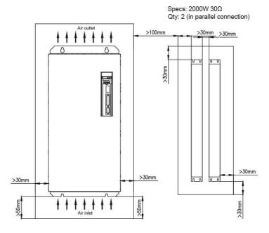
Figure 10-2 MH860-150/170/180/215 drive and braking resistor layout (mm)
