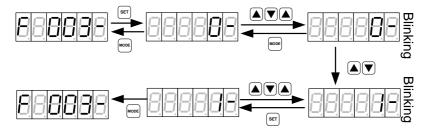
For calibration commands, such as pressure linear zero calibration, after the setting: if the LED displays 0, the calibration succeeds; if the LED always displays 1, the calibration failed.
