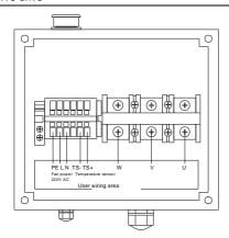
Figure 4-8 Motor wiring terminals
