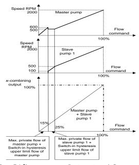
Figure 7-1 Slave pump responding to master node flow commands
