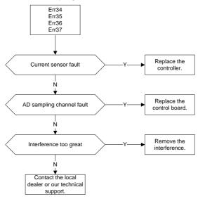
Err38: DC voltage sampling fluctuation fault
