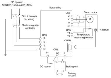
Figure 4-10 Wiring diagram of >=110kW main circuit
