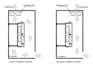
Figure 3-2 Ventilation fan installation position
