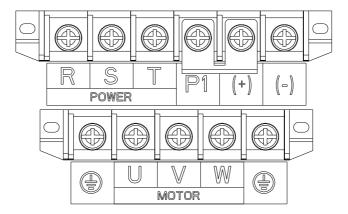
Figure 4-5 Terminal diagram of the 110kW main circuit
