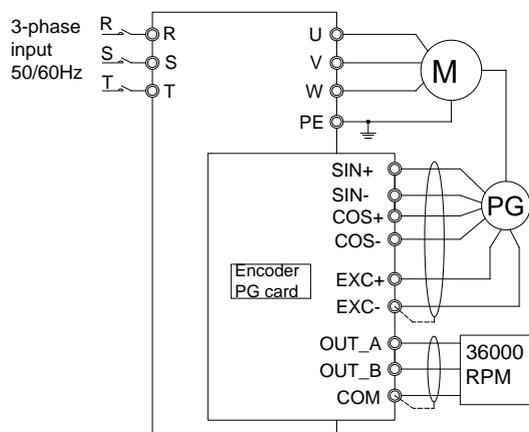
Figure 11.11 Wiring diagram of rotary encoder PG card
