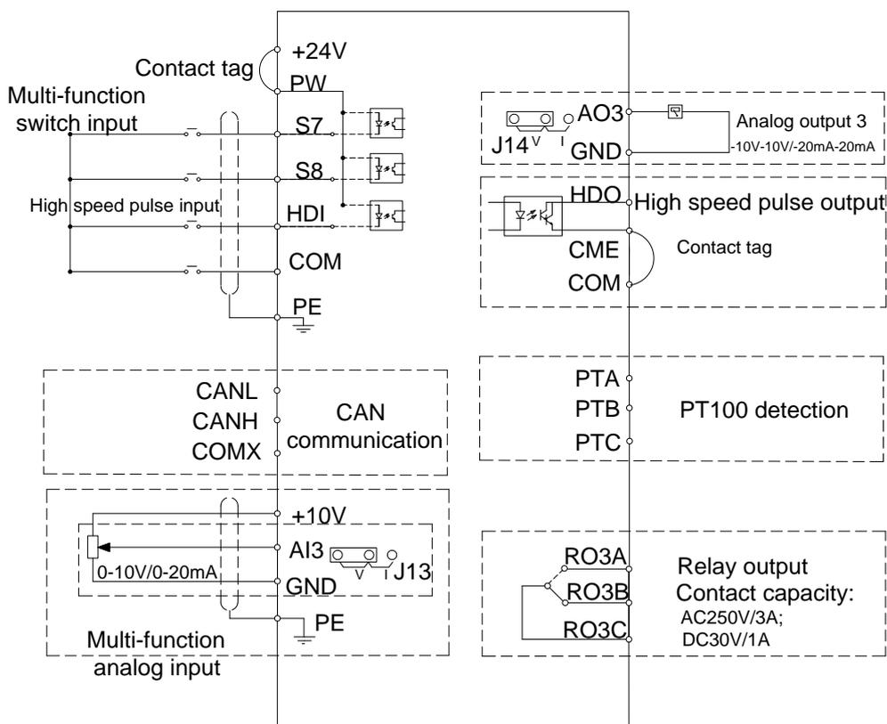
Figure 11.2 Wiring of Goodrive3000 comprehensive extension PG card
