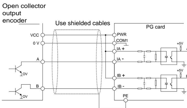
Figure 11.5 Wiring diagram of open collector output encoder
