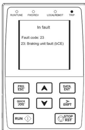
If the VFD detects the fault signal, it will enter into the fault pre-alarm displaying state. The keypad will display the fault information. The TRIP LED on the keypad is on, and the fault reset can be operated by the STOP/RST on the keypad, control terminals or communication commands.
