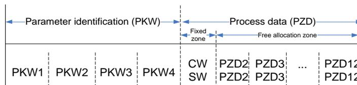
Figure 9.8 PROFIBUS-DP packet structure
