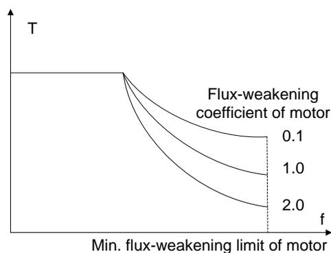
P03.22 and P03.23 are valid at constant power. When the motor runs above the rated rotating speed, it comes into weakening state. The curvature of weakening curve can be changed by modifying the control coefficient. The larger the coefficient is, the steeper the curve is.
