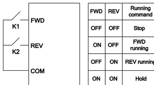
1: 2-wire control 2: Separate the enable from the direction. FWD defined by this mode is the enabling one. The direction depends on the state of the defined REV.
