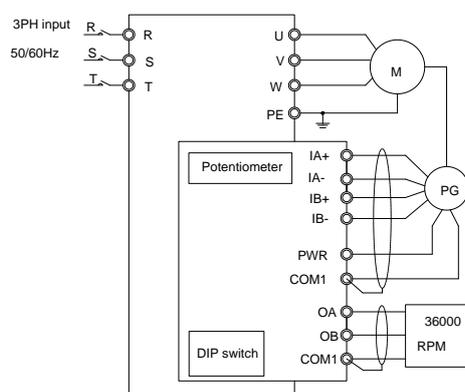
Figure 11.3 Wiring diagram of incremental encoder PG card
