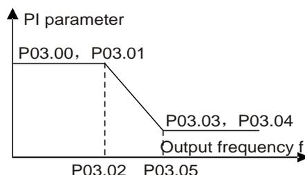
The speed loop dynamic response characteristic of vector control can be adjusted by setting the proportional coefficient and integral time of the speed regulator. Either increasing proportional gain or decreasing integral time will speed up the dynamic response while too high proportional gain or too low integral time will easily cause system oscillation and overshoot. Too low proportional gain will also easily cause system oscillation and speed static deviation.
