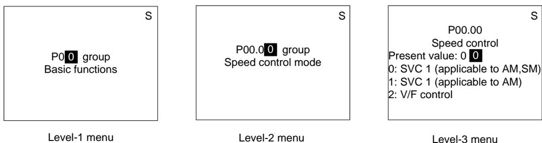
Figure 4.2 Operation flow chart of three levels menu
