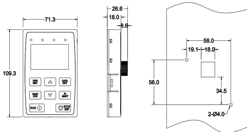
Figure 4.3 LCD keypad dimension
