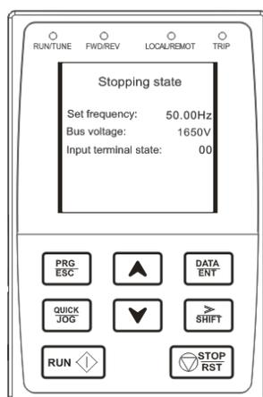
When the VFD is in the stopping state, the keypad will display stopping parameters which is shown in figure.
