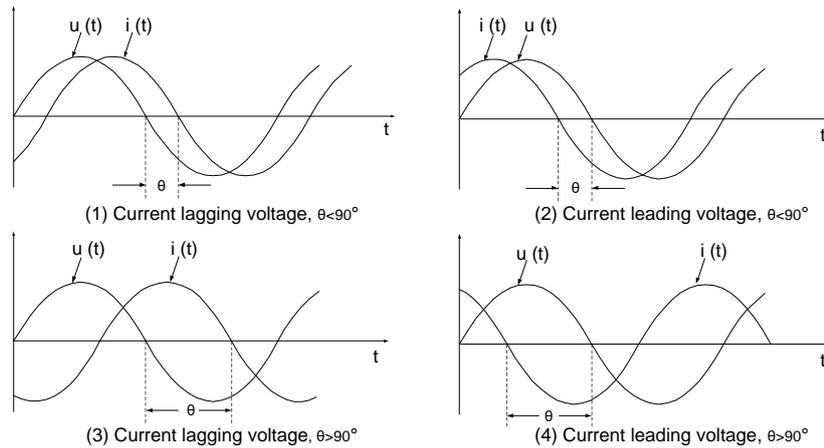
Figure (1) and (3) corresponds to inductive and figure (2) and (4) corresponds to capacitive.
