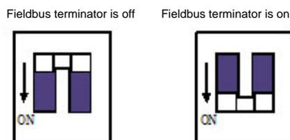
Figure 9.3 Fieldbus terminator
