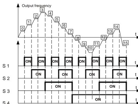
When S1=S2=S3=S4=OFF, the output way of the frequency is selected by the function code P00.06 or P00.07. When not all S1=S2=S3=S4 terminals are off, the VFD runs at multi-step speed and the multi-step speed has the priority over the keypad, analog values, high-speed pulse, PLC and communication frequency input. Select at most 16-step speed via the the combined codes of S1, S2, S3 and S4.
