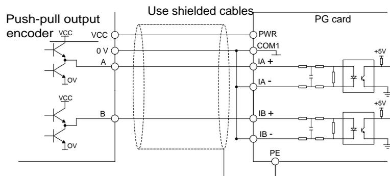
Figure 11.6 Wiring diagram of push-pull output encoder
