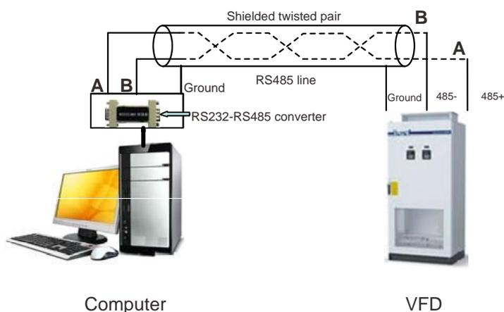
Figure 8.1 RS485 physical connection in single application
