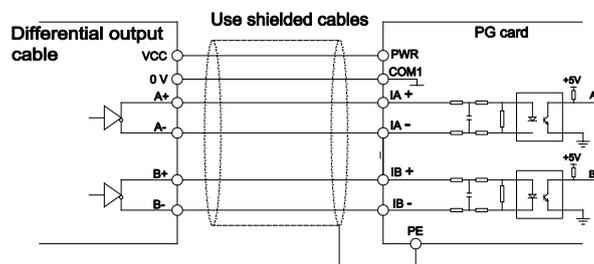
Figure 11.4 Wiring diagram of differential output encoder
