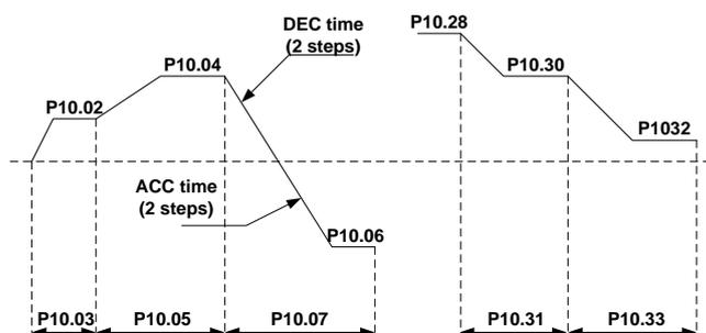
Multi-step speed can be set continuously in the range of  $-f_{max}$ – $f_{max}$
