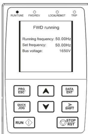
After the VFD receives valid running commands, the VFD will enter into the running state and the keypad will display the running parameters. RUN/TUNE LED on the keypad is on, while the FWD/REV is determined by the current running direction which is shown in figure.
