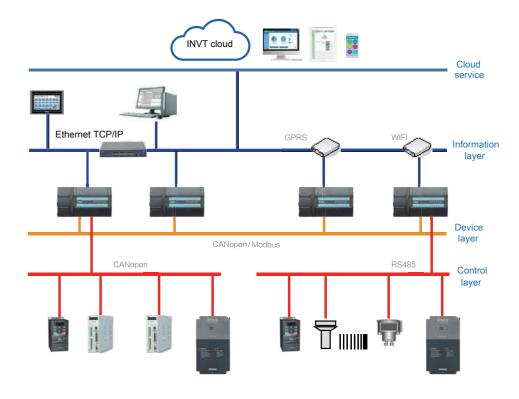
Communication network covers IoT, control communication and device communication network to realize inter-connection among information layer, control layer and device layer.
