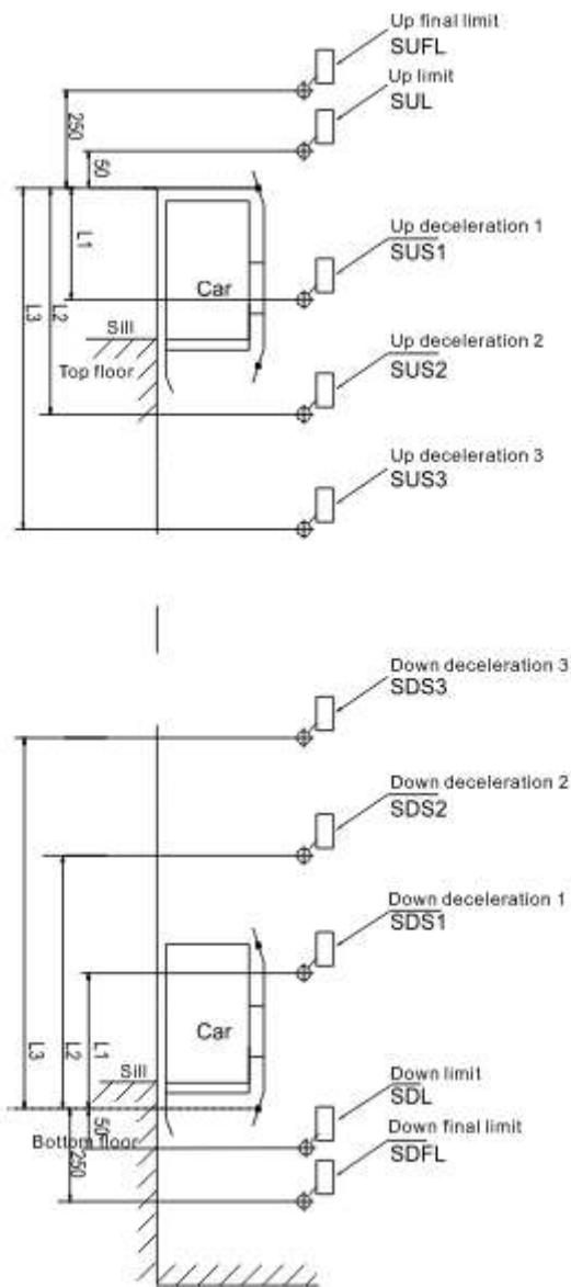
Figure 4-10 Installation position of the hoistway switch
