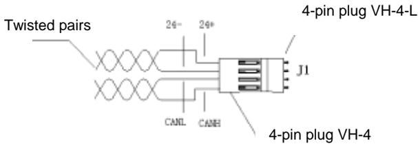
Figure 10-2 connection of the car main controller DC-01
