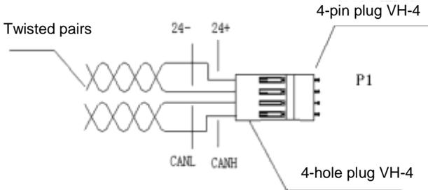
Figure 10-13 Connection between calling display board, power and communication bus
