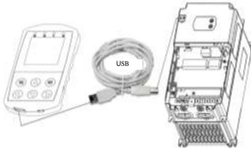
Figure 5-1 Connection of manual operator interface with EC100
