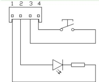
Figure 10-5 Connection of P1-P8 command button wires
