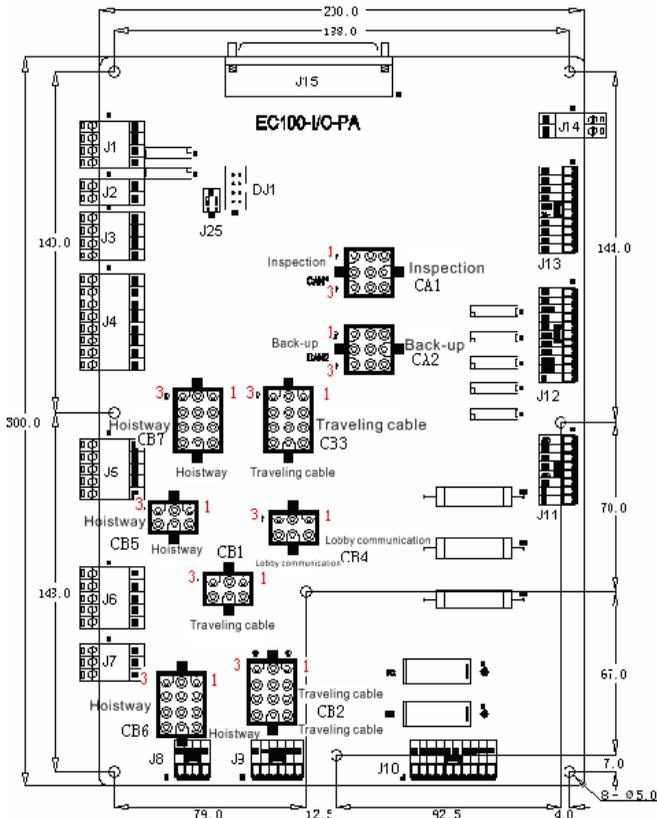
Fig 4-7-2 Appearance and terminal layout of EC100- I/O-PA
