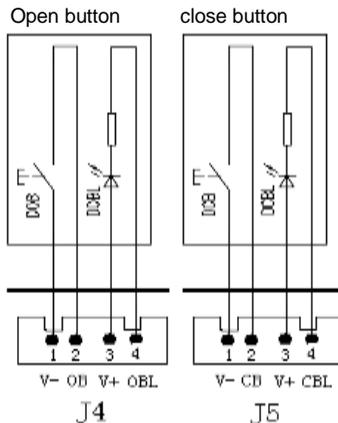
Figure 10-3 Connection of door button and indicator
