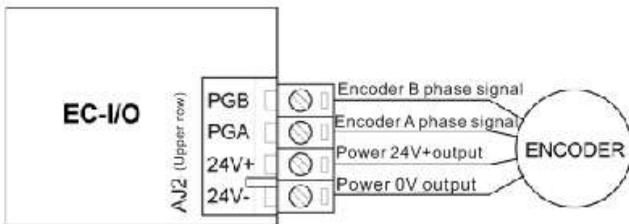
Figure 4-8 Wiring of asynchronous master encoder
