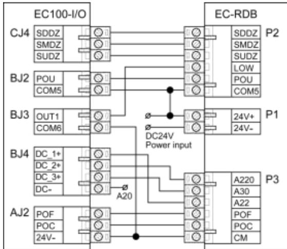
Figure 10-28 Wiring diagram of EC-RDB and peripheral interface
