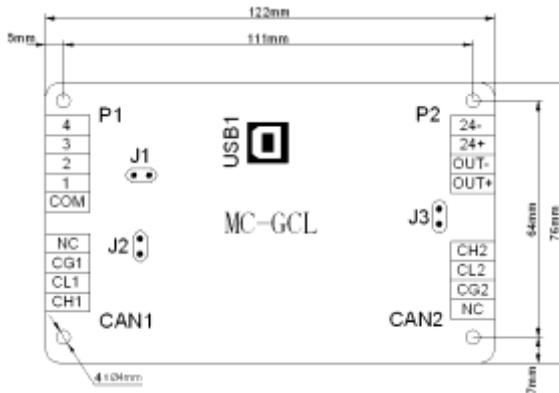
Figure 10-23 Installation dimension
