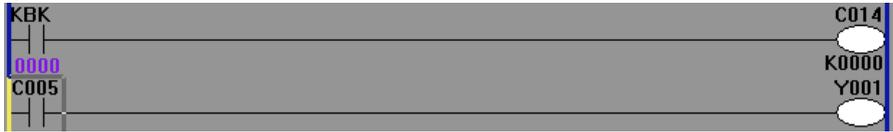
The figure above means output Y001 when the accumulative opening times of the braking unit reach 2000.
