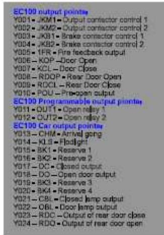
The main board provides two programmable output relay OUT1 and OUT2 for the sub-development. The others are non-programmable.
