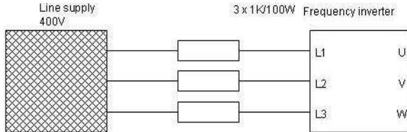
Figure 11-1 400V charging circuit of the drive device
