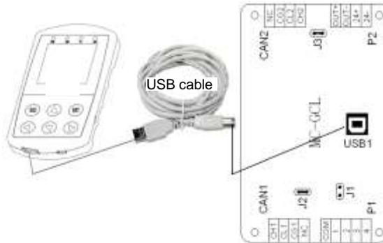
Figure 10-25 Connection of manual operator and MC-GCL
