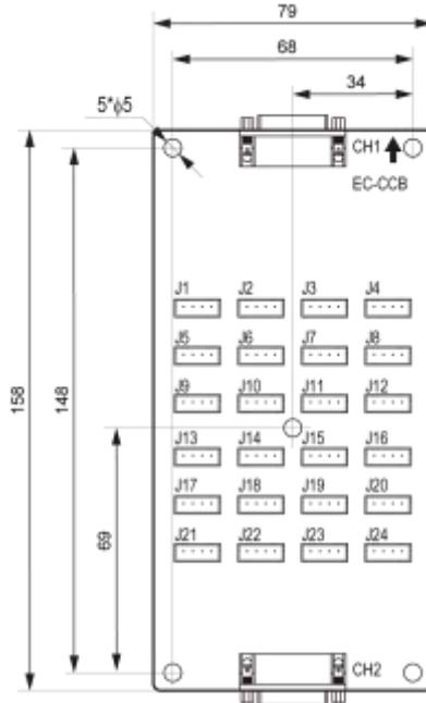
Figure 10-19 Installation dimension
