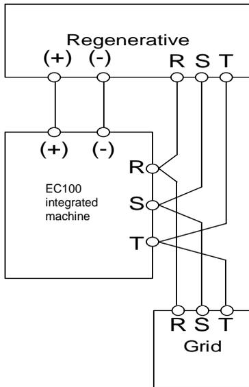
Figure 4-6 Connection diagram of the energy feedback unit
