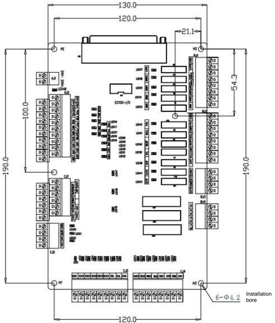
Figure 4-7 Appearance and terminal layout of I/O board
