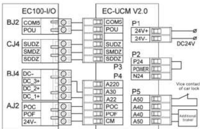
Figure 10-30 Wiring diagram of EC-UCM and peripheral interface
