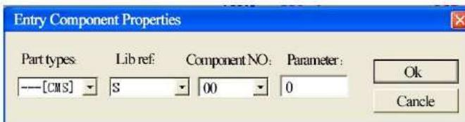
Speed comparator S, when SXX is larger than the set parameter (XX is any one of the component code in 00-07), the unit of the parameter is mm/s
